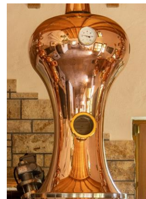
Kothe – Whisky helmet With increased copper surface and smooth expansion of the spirit
